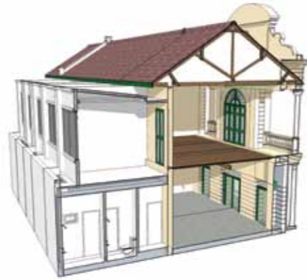
Figure 15. Rehabilitation was chosen as the treatment for the Na Phralan shophouses as there is an extended structure at the rear to meet contemporary use (source: CPB and Kudakan Co. Ltd)
